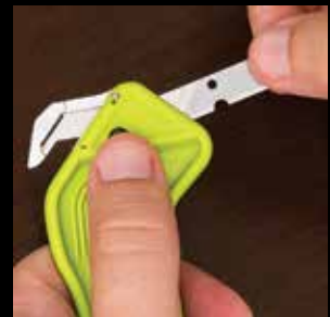
While holding the blade release button down insert a new blade and carefully slide into slot
