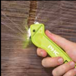
Hold film taught with opposite hand and cut downward
